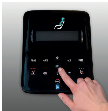
Fig. 4. The demonstrator for the control panel of a center console with inductive button functions was produced in the DC process using back injection molding of a printed Makrofol PC film, and the surface was finished with a puroclear-based deep gloss
